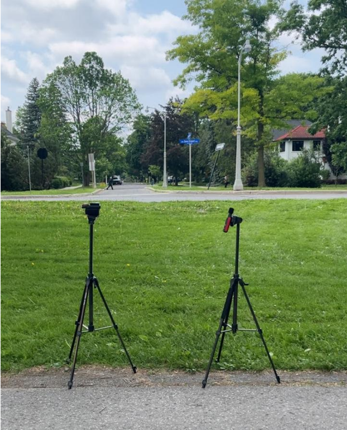
Figure 4: Equipment setup at a sampling location for noise (right side), PM2.5, and UFP (left side) measurements. (Photo credit: Farès Chéraitia)
