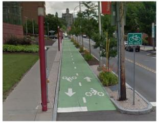
Add tactile feedback at driveways. Adding temporary speed bumps or full grade separation would slow turning vehicles.
